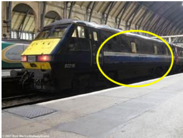
Figure 13 Driving Van Trailer: Space for the Carriage of Goods
