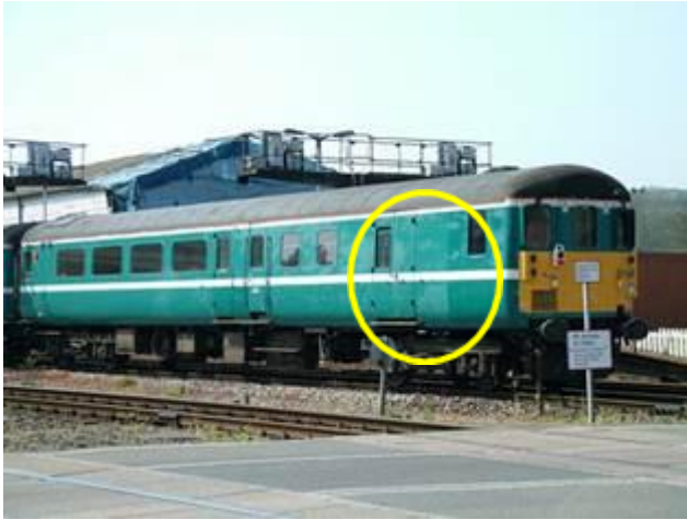
Figure 14 Other Driving Van Trailer: Space for the Carriage of Goods
